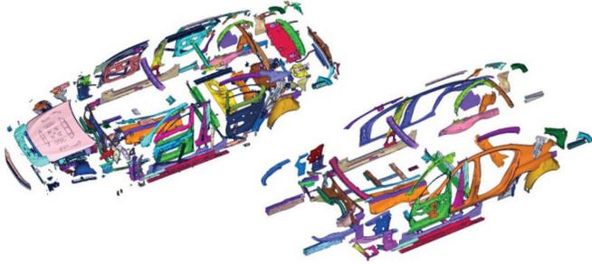
Figure 2. Modeling potential sheet metal failure during a crash test simulation is standard practice at BMW Group. The figure on the left shows the typical body components where this is considered. The effects of prior forming processes, such as stamping, can have an influence on failure, and the figure on the right shows the typical components where results from earlier forming simulations are mapped onto their crash model counterparts.
