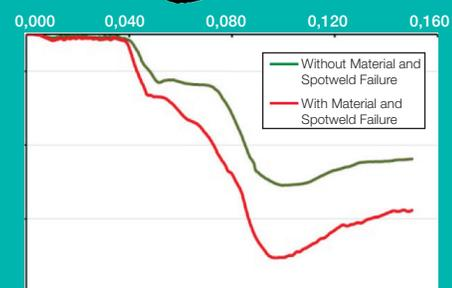
Frontal offset crash test simulation in Abaqus FEA (top) and corresponding firewall intrusion results with and without local failure mechanisms incorporated in the model (bottom).
